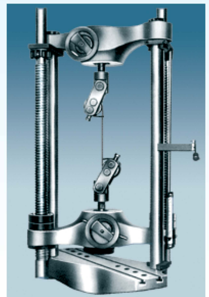
Attachment for Tension Test for Wire Ropes
